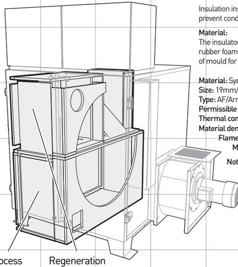
Insulation installed inside of process air inlet and/or regeneration air inlet to prevent condensate forming on the outside of the unit.
