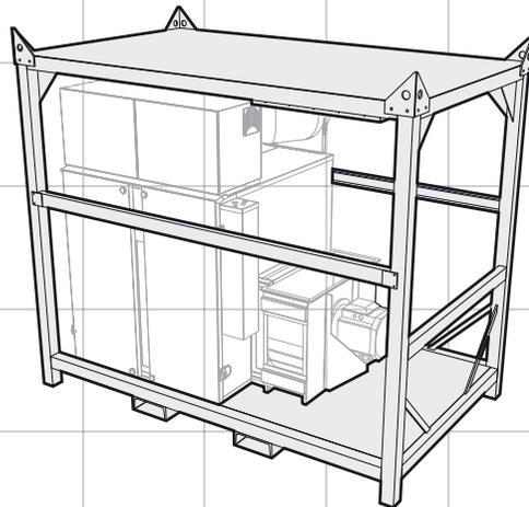
Unit fixed inside a welded steel frame to facilitate transport and instantly set up the unit for operation.
